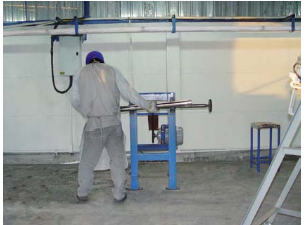
HAND POLISHING LAND ROVER DEFENDER ROLL BAR 76 MM
