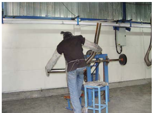
HAND POLISHING LAND ROVER DEFENDER ROLL BAR 76 MM
