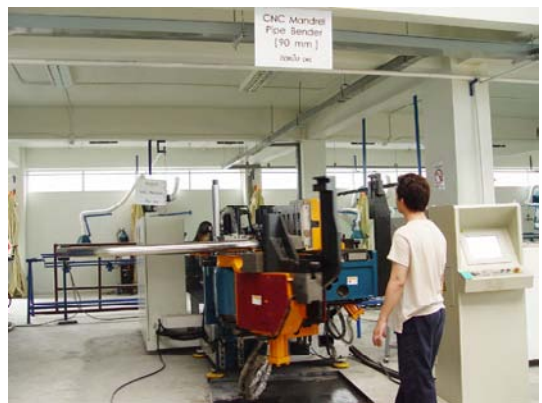
5 axis 90 mm CNC Mandrel Tube Bender
