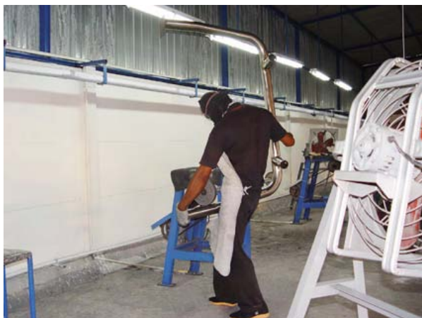
HAND POLISHING LAND ROVER DEFENDER ROLL BAR 76 MM
