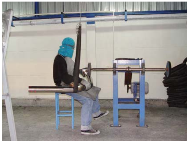
HAND POLISHING LAND ROVER DEFENDER ROLL BAR 76 MM
